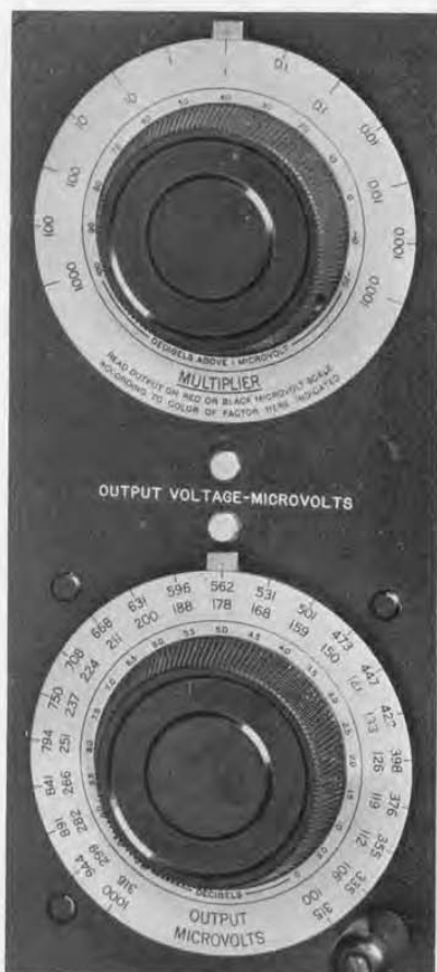
FIGURE 3. Output voltage controls for the TYPE 600-A Standard-Signal Generator. The dials are now set for 178 microvolts or 45.0 db above a reference level of 1 microvolt. If the upper dial were moved clockwise one division, the output would be 562 microvolts or 55.0 db
