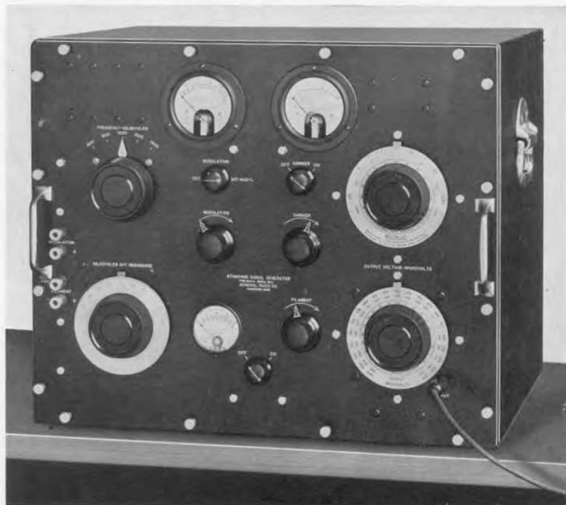
FIGURE 1. Panel view of the TYPE 600-A Standard-Signal Generator. At the upper left is the channel selection switch and immediately below it the selectivity or "kilocycles-off-resonance" control. At the right is the two-stage attenuator shown in detail in Figure 3 and to the left of it the voltmeter for indicating attenuator input
